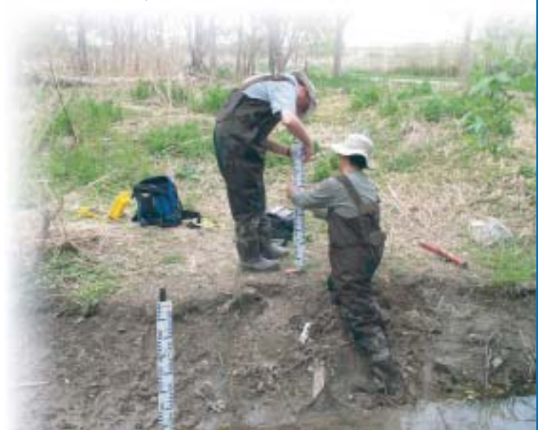
CVC crew installing staff gauge for high flow events.
